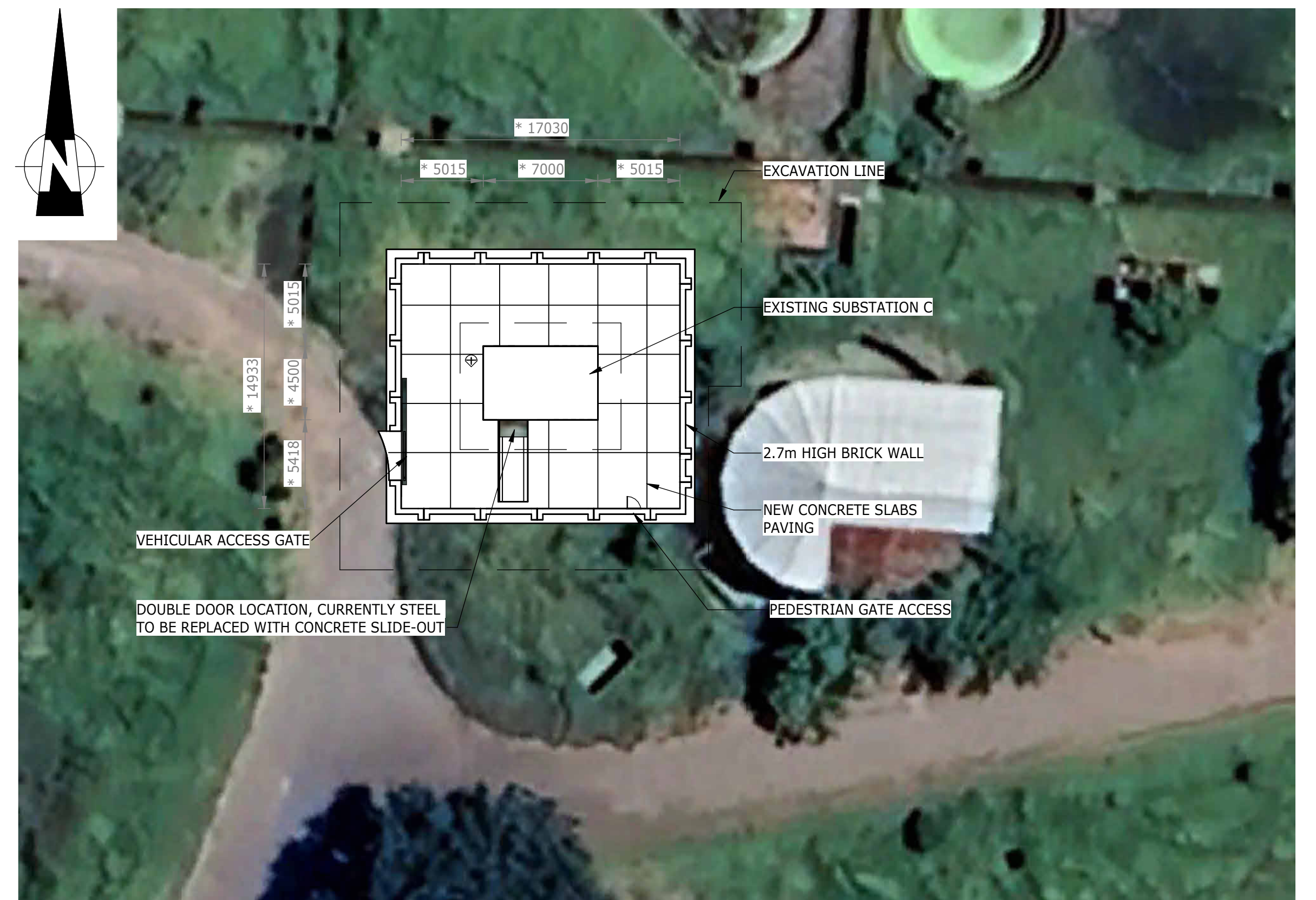
PLAN VIEW SUBSTATION C
