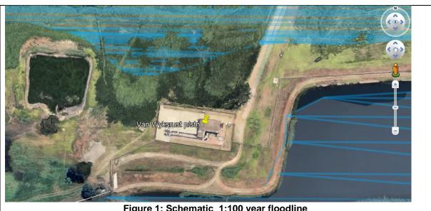
Figure 1: Schematic 1:100 year floodline
