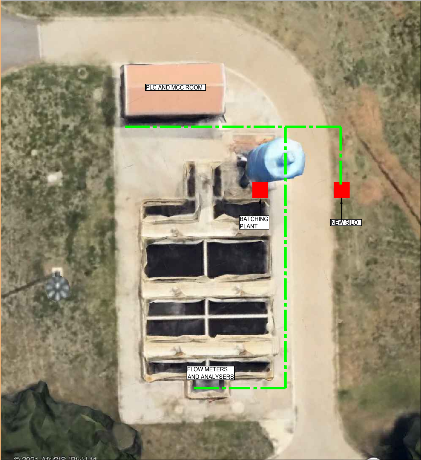
LIME PLANT CABLE ROUTE
