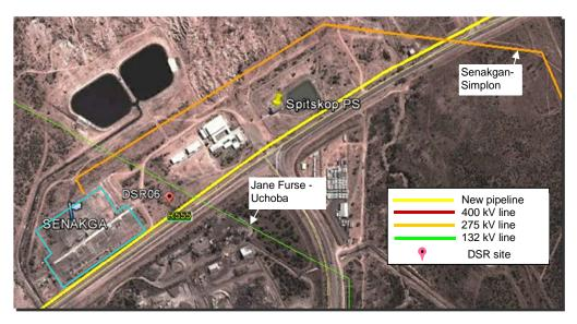
Figure C.2 - Pipeline route detail near Senakgangwedi substation
