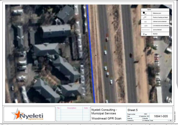
The images above shows that there are verious services crossing the path of the pipeline, a AutoCad co-ordinated drawing has been provided.
